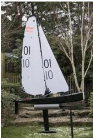
and to windward the balance was all the place, almost unsailable. I didn't want to go any deeper than the DF65 fin so we need to find out how wide it needed to be to work in light winds, but narrow enough to minimise drag downwind. Dave Creed helped out here by moulding a couple of aerofoil section sleeves that slid over the fixed DF65 metal keel, they were fairly crude but easy enough for us to keep trimming down until we seemed to have the
